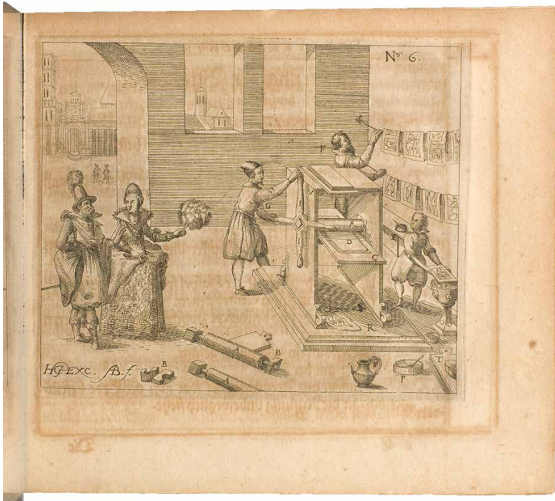
Fig. 4. Anonymous, Plate printer , etching, in Heinrich Zeissing, Theatri machinarum , pt. 3, 2nd ed., Leipzig, Gross, 1613, fig. 6; Wolfenbüttel, Herzog August Library, department of photography.
